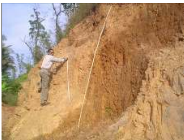
Fig. 2. A deeply weathered Red soil profile which is located near the Malnaad (Kodigibail) basins. The depth of the soil profile is in excess of 2 m depth and preferential wetting is also evident. Weathered rock is also visible in the right bottom corner.
