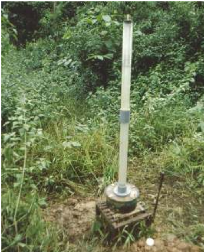
Figure 4-8: Infiltrometer used to measure soil infiltration rates in Aghanashini
