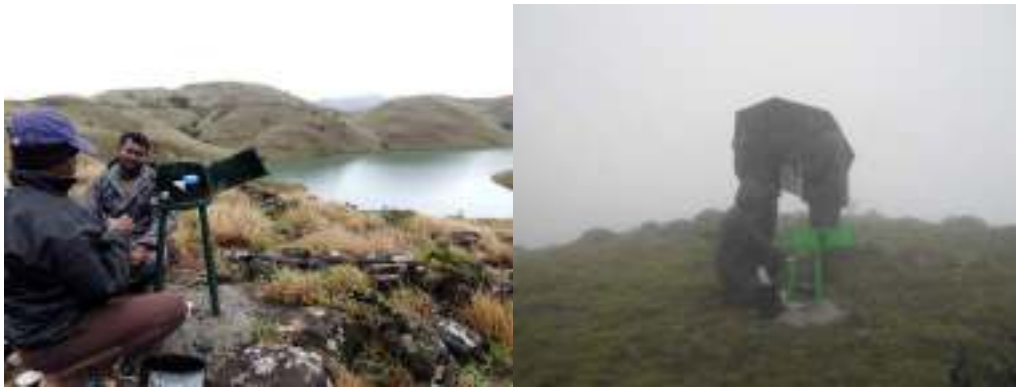
(b) Downloading data from rain gauges overlooking the Upper Bhavani reservoir and at Kolaribetta.
