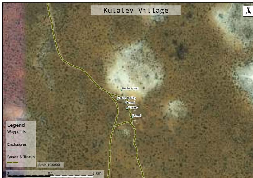
**Figure 10:** A mosaic of Google Map based satellite imagery of Kulaaley village with some landmarks, enclosures and roads digitised. The former were collected with a handheld GPS unit. The source data is scaled to 1:5000 which conforms to a cadastral scale and allows users to mark and identify features easily visible on the satellite image.
