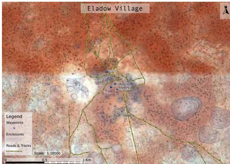
**Figure 8:** A mosaic of Google Map based satellite imagery over the Eladow village with some landmarks, enclosures and roads digitised. The former were collected with a handheld GPS unit. The source data is scaled to 1:5000 which conforms to a cadastral scale and allows users to mark and identify features easily visible on the satellite image.
