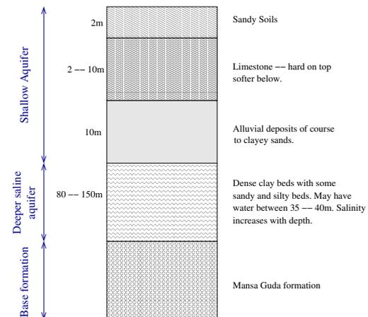
**Figure 4:** A diagrammatic view of the Merti aquifer based on (Krhoda, 1989). The shallow aquifer with its fractures and sink-holes provides an opportunity to recharge it locally.
