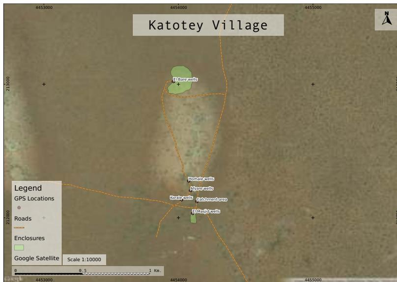
**Figure 16:** A mosaic of Google Map based satellite imagery over the Katotey village with some landmarks, enclosures and roads digitised. The former were collected with a handheld GPS unit. The source data is scaled to 1:5000 which conforms to a cadastral scale and allows users to mark and identify features easily visible on the satellite image.
