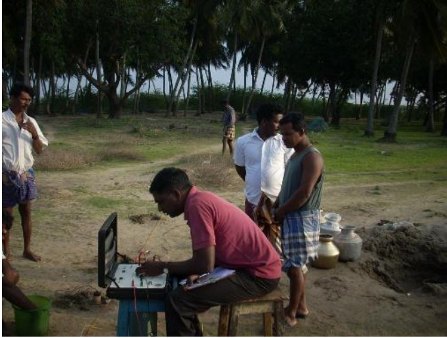
Figure A.1.: Electrical resistivity test underway.
