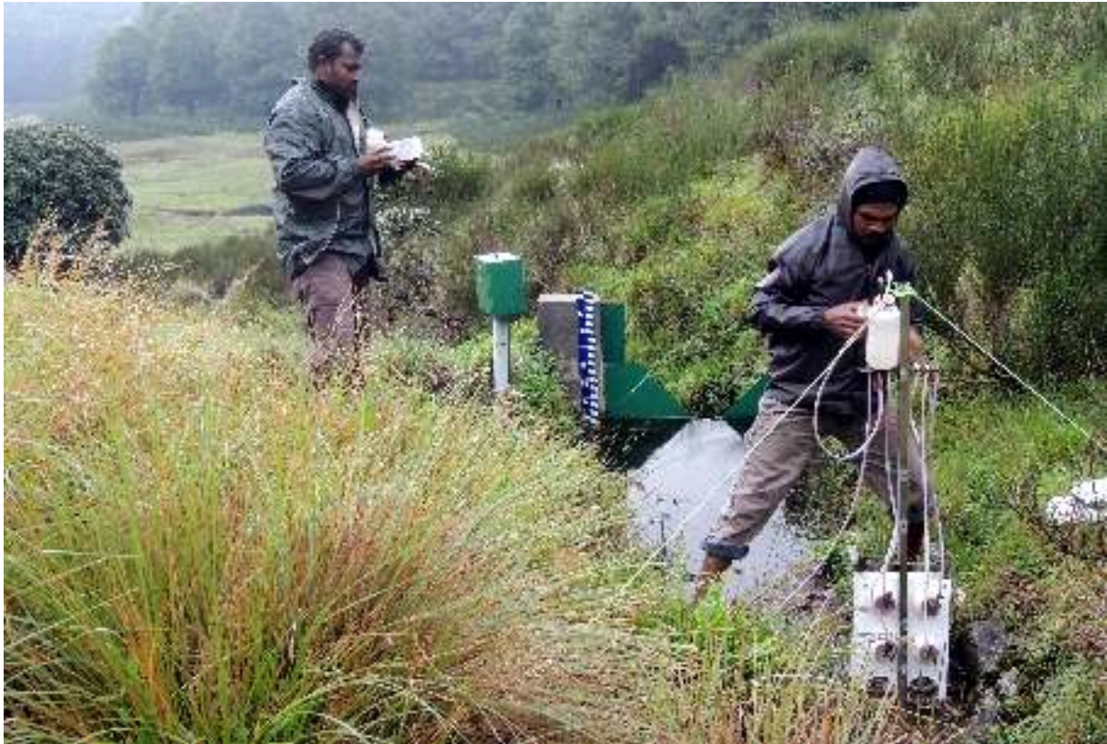
Water samples being collected from a weir installed downstream of a wattle ( Acacia mearnsii ) dominated catchment. The wattle is scheduled to be removed under the grassland restoration programme. We hope to be able to quantify the ensuing changes in stream-flow and the quality of the runoff.
