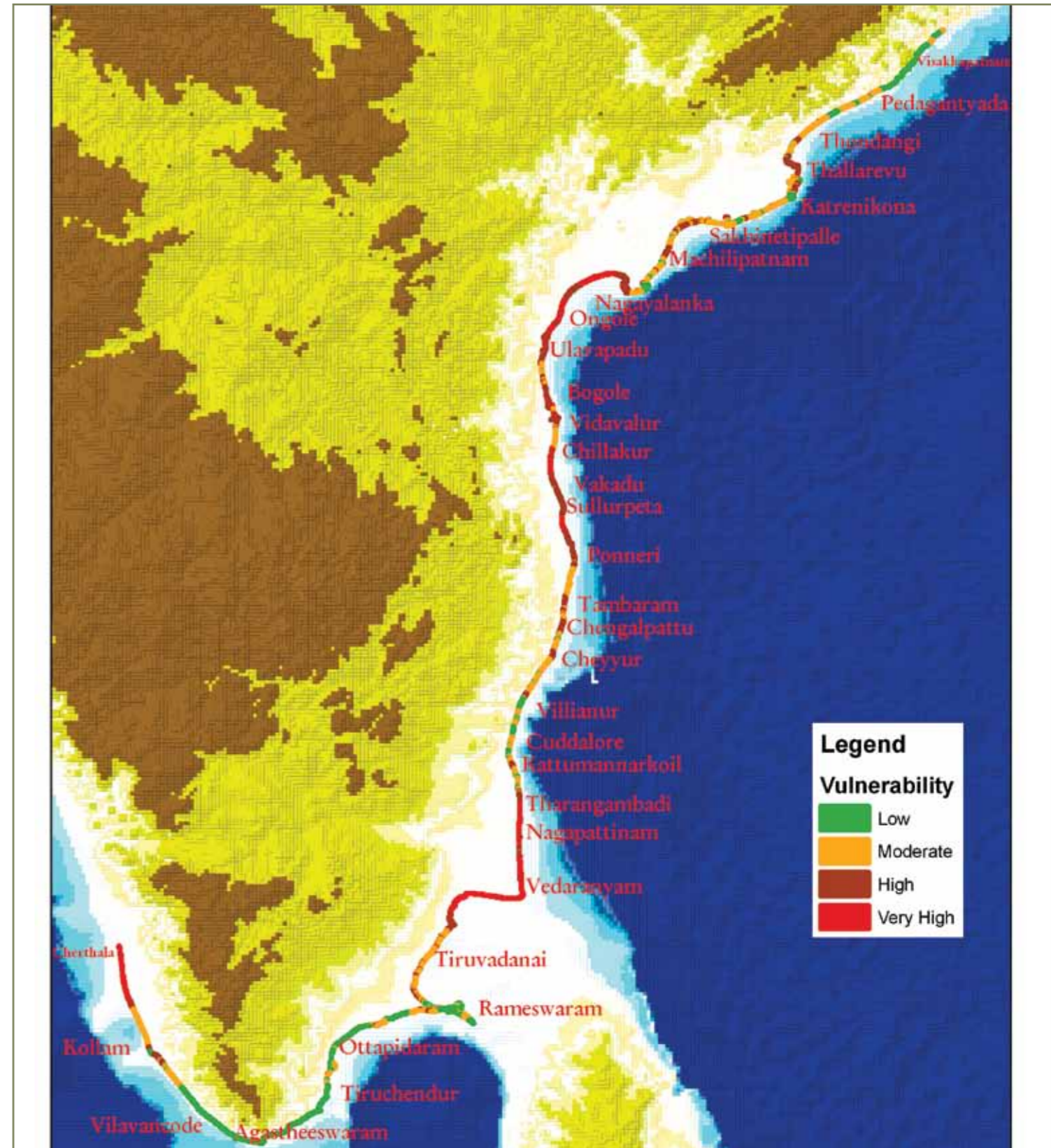
Coastal vulnerability map of the southern coast of India which incorporates coastal erosion/accretion rates, geomorphology, wave energy, tidal range, topography and bathymetry.
