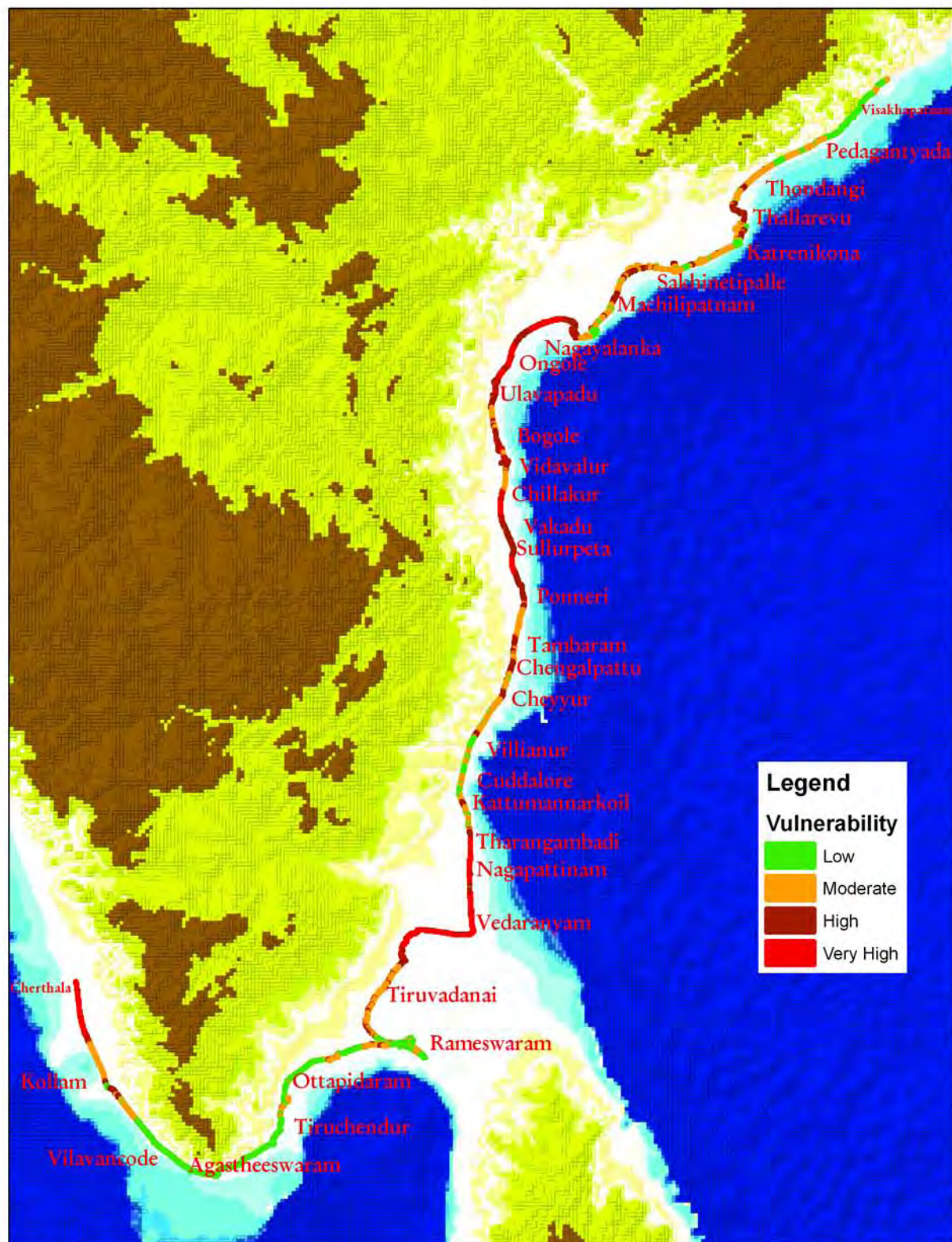
Figure 2.10: Coastal Vulnerability map of the southern coast of India which incorporates coastal erosion/accretion rates, geomorphology, wave energy, tidal range, topography and bathymetry.
